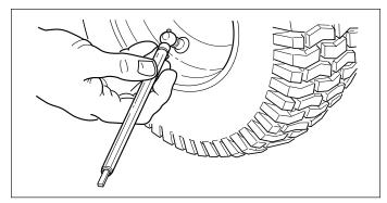
Figure 6. Checking Tire Pressure
